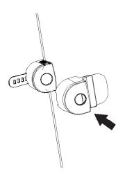
Press outer cover against outer glass panel to hold in place and pull adhesive tab. Press and hold adhesive against outer glass panel for 10 seconds.
