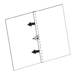
To lock the L410 slide the glass panels closed. The L410 will self latch into the locked position.
