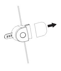
Use screw driver provided to tighten set screw on outer cover. Do not over tighten.
